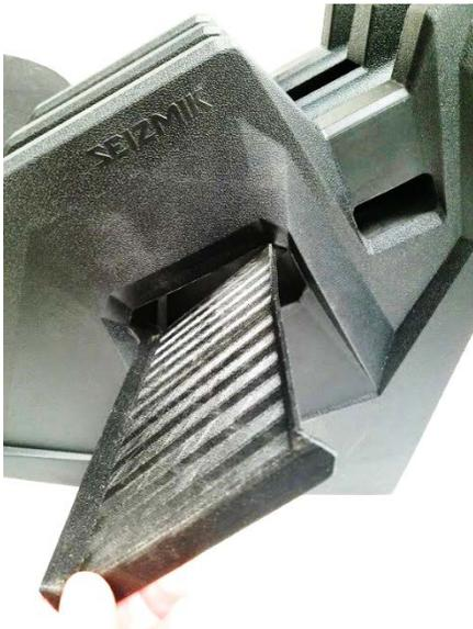
1. Start by Installing the plastic Seatbelt insert by placing it through the large center hole.
