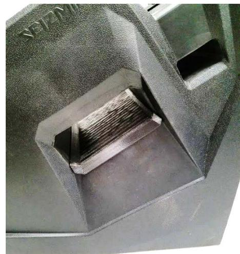
2. When installed, the seatbelt insert should lay flush and match the style lines of the foam base.
