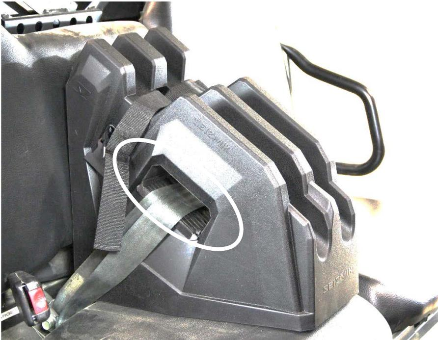
5. Place the assembly on the vehicle seat. Run the seat belt through the middle hole and buckle into the seatbelts receptacle. Pull the loose tab to get the seatbelt as tight as possible.
