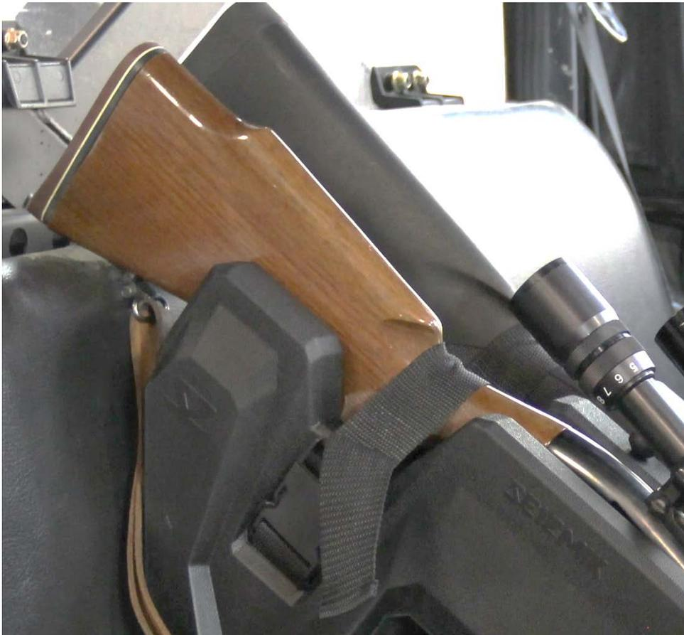
6. Place gun into channel as pictured above. Buckle the gun hold down strap and pull tight. For best results, place the gun hold down strap in the notch on the stock (seen above).
