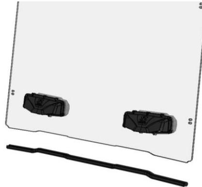
2. Push the gasket on the bottom of the windshield with the bulb section oriented as shown
