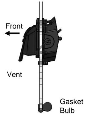
3. Snap 2 clamps on each side of the roll cage and 2 across the top with the flanges facing forwards. Insert bolt through backing plates and windshield and loosely install nuts on all 6 clamps. Adjust windshield as needed and tighten nuts.
