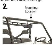
The Pro-Fit and Defender mirror clamp mounts to the middle of the bent sheet metal cross bar.
