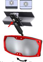
Line up the mirror with arm attached and install using M8 x 25mm socket head bolt. Adjust mirror as necessary.
