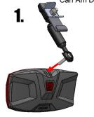
Screw Mirror Arm into Mirror using M8x20mm button head bolt.
