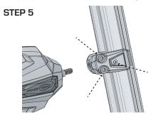
Remove mirror housing from the clamp. Tighten all clamp boltst
