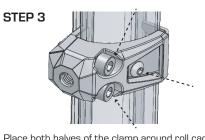
Place both halves of the clamp around roll cage tube. Complete the clamp assembly by tightening bolts. **DO NOT TIGHTEN THEM ALL THE WAY YET.**
