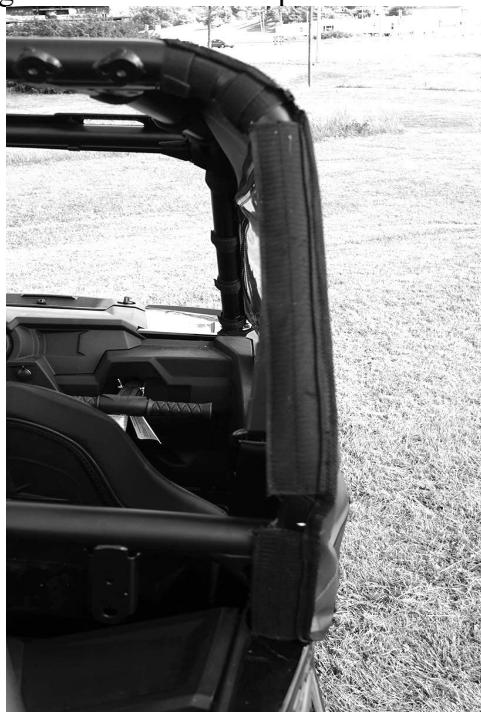
5. Lastly snap the bottom of the door to the plastic doors on the RZR. NOTE: it helps to place the screw snaps into the sockets on the cabs first, then starting at the top one, push them into the plastic so a small dimple is left behind. Then pull the screw snap back out and screw it into the plastic where the mark was made. See photo below
