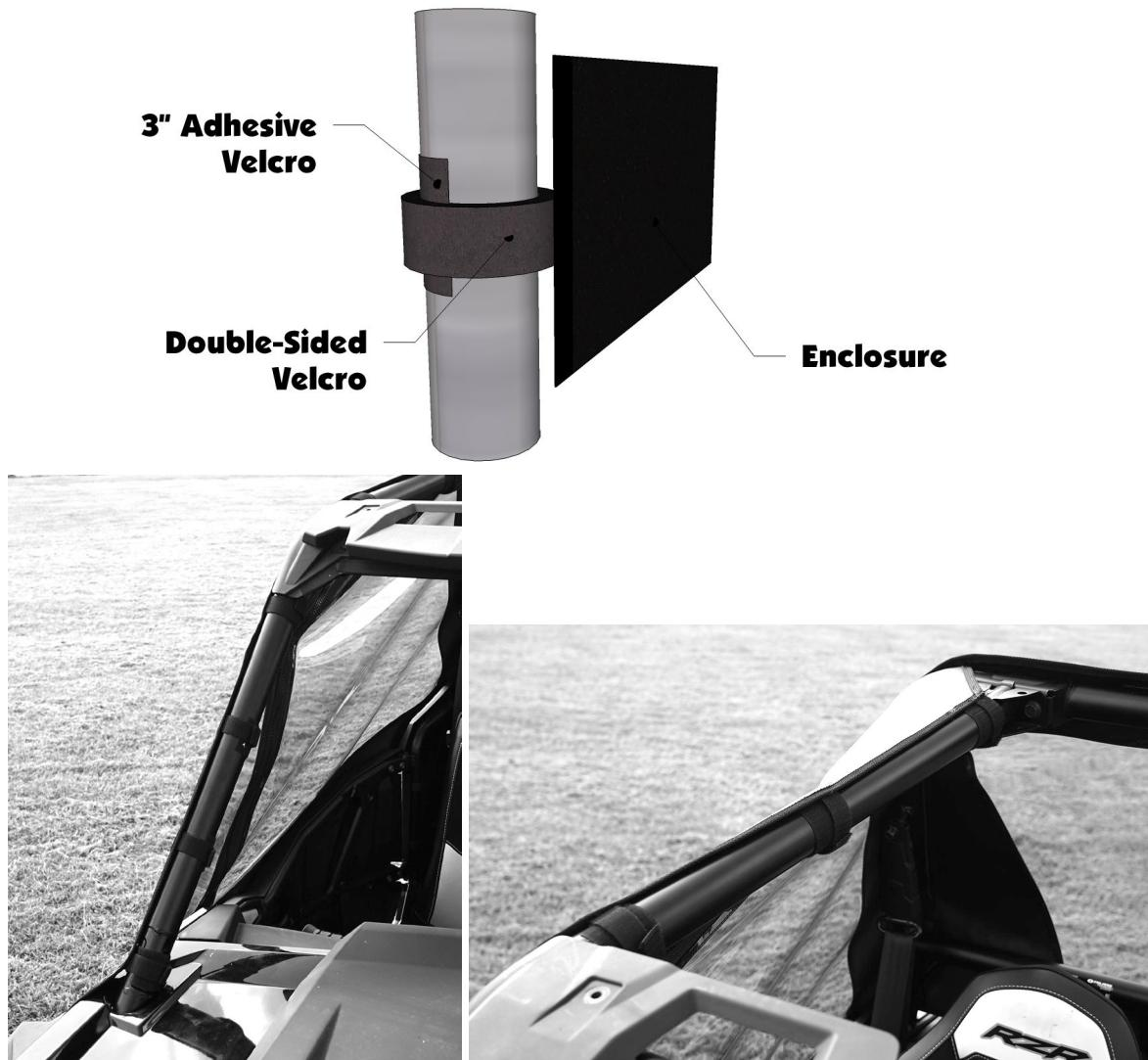
4. After installing the double-sided strips move to the rear of the door and attach the two Velcro tabs to the rear bar using the corresponding adhesive Velcro strip. See Photo Below:
