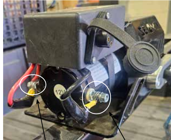
Control box positive (red) connection terminal
