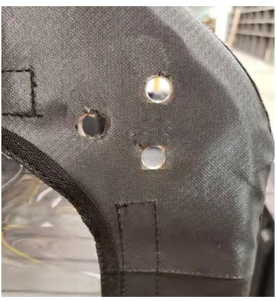
9. Holes need to be cut in door textile panels in order to mount the Upper and Lower Sliding Hinges. Ensure textiles are tight and fit as desired before marking and cutting holes. Take a sharp scribing tool and punch a small hole through the textile indicating the center of the slot. Take a razor blade and carefully cut out the small amount of textile so that the supplied M8 bolt may pass through the plate and the textile. Repeat this process for the lower mounting location.
