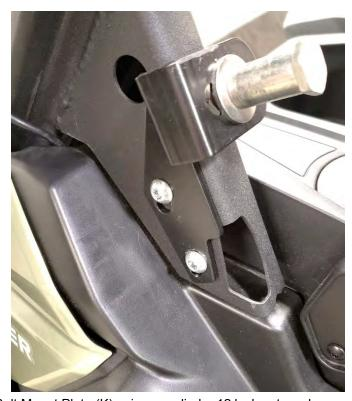
13. If not already done so, attach Striker Bolt (L) to Striker Bolt Mount Plate (K) using supplied m12 lock nut as shown.
