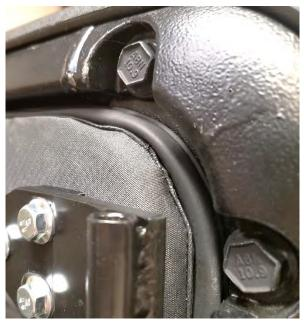
**16.** Adjust the door in and out using the slots in the Upper Door Mount (H) and Lower Door Mount (I). Use these slots to increase or decrease compression on the door gasket. See images above for proper gasket compression
