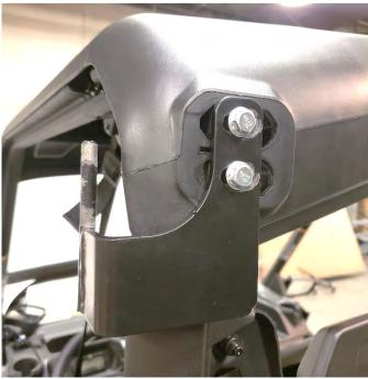
3. Locate the 2 threaded holes at the top of the cab where the roof mounts. Remove factory mounting hardware to expose the threaded holes. Install Upper Door Mount (H) using 2 M8x16mm flange head bolts. Snug the bolts down but do not tighten all of the way. You will need to adjust them later once the door is on.
