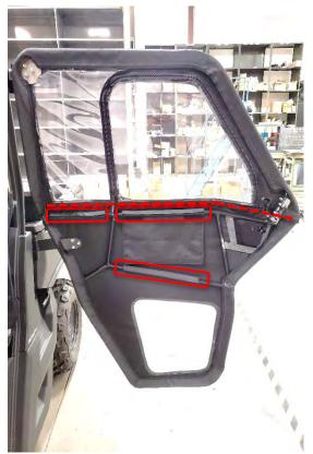
**4.** The upper and lower textiles come on each half of the frame but you will need to attach the halves together and ensure they are properly secured. The highlighted areas are the main areas you will need to address. There are 3 center flaps that wrap around the tubing along with the 2" Velcro seam between the upper and lower textiles.
